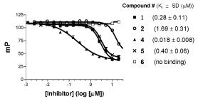
**Figure 4.** Competitive binding curves of small-molecule inhibitors to Mcl-1 as determined in our fluorescence-polarization-based Mcl-1 binding assay using a fluorescently tagged Bim peptide as the tracer (Supporting Information).
