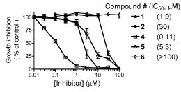
**Figure 6.** Inhibition of cell growth by designed small-molecule BH3 mimetics in the MDA-MB-231 (2LMP) breast cancer cell line. Cells were treated for 4 days and cell growth was determined using WST-based assay.
